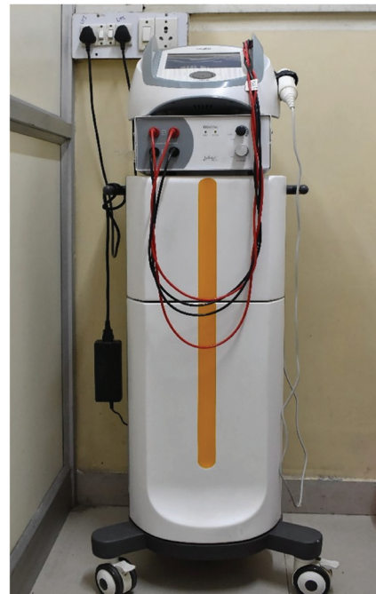
Figure 2. TENS machine TENS, transcutaneous electrical nerve stimulation.
